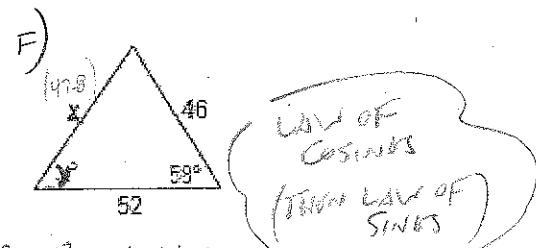
$$\begin{aligned} x^2 &= 52^2 + 46^2 - 2(52)(46)\cos 58^\circ \\ x^2 &= 2704 + 2116 - (4784 \cos 58^\circ) \\ x^2 &= 4820 - (2535.13376) \\ x^2 &= 2284.86624 \\ x &= 47.8 \end{aligned}$$
