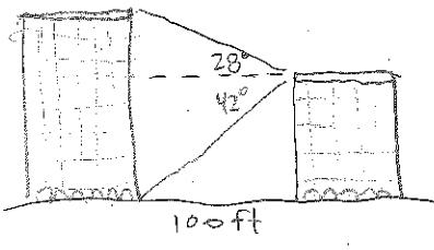
$$\begin{aligned} \tan 28^\circ &= \frac{x}{100} \\ x &= (100)(\tan 28^\circ) \\ x &= 53.2 \text{ feet} \end{aligned}$$
